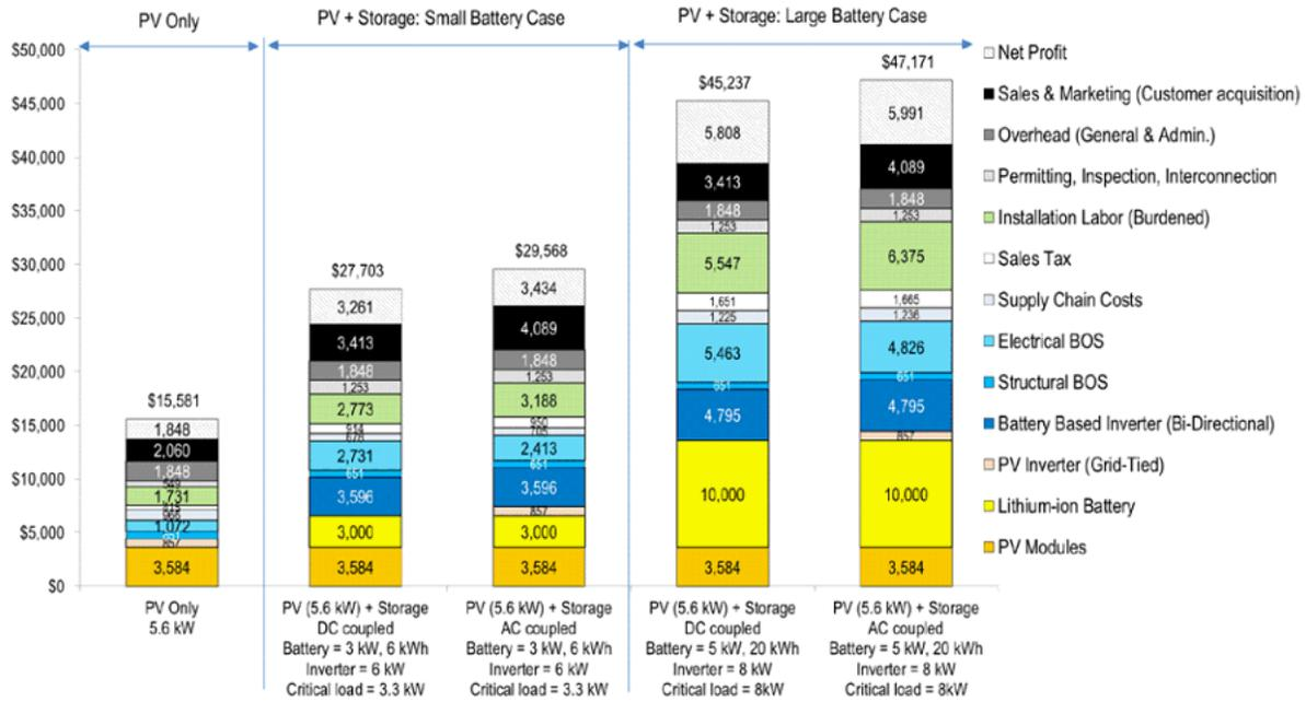
Figure 3. Modeled total installed cost and price components for residential PV-plus-storage systems, small-battery case vs. large-battery case (2016 U.S. dollars)
